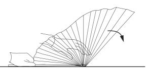
④ Hold the fan holder (Part C) and lampshade (Part D) with your one hand. Press the lampshade flat on the table with your other hand.
