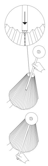
Slide the fan holder (Part B) all the way down on the stitching track. ③ Place the fan holder (Part B) with the attached lampshade (Part C) on a table, with the flat side of the fan holder facing downwards.
