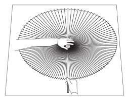
Screw the top cover (Part F) onto the fan holder (Part B).
